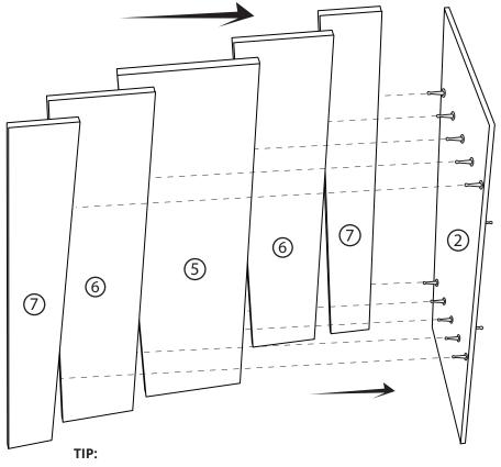
Because of the tight space between each divider it is easier secure one panel at a time, allowing room to get to the Camlocks easily. Note: the last panel 7 will need a short screwdriver to get to the Camlock.
